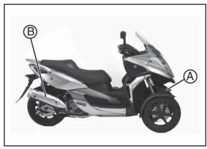
B - Heat shield on the exhaust pipe.
